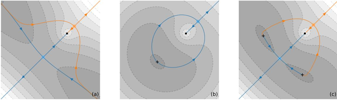
Figure 3: Examples of a single well in uniform areal recharge. The head contours for the background flow are shown in Figure 2. Equipotentials (filled grey contours, darker grey is higher potential), capture zone envelopes (colored), stagnation points (light colored dots), and high points (crosses) for a well in background flow that is (a) linear recharge for flow in direction  $\alpha = \pi/4$ , (b) circular recharge, and (c) elliptical recharge.
