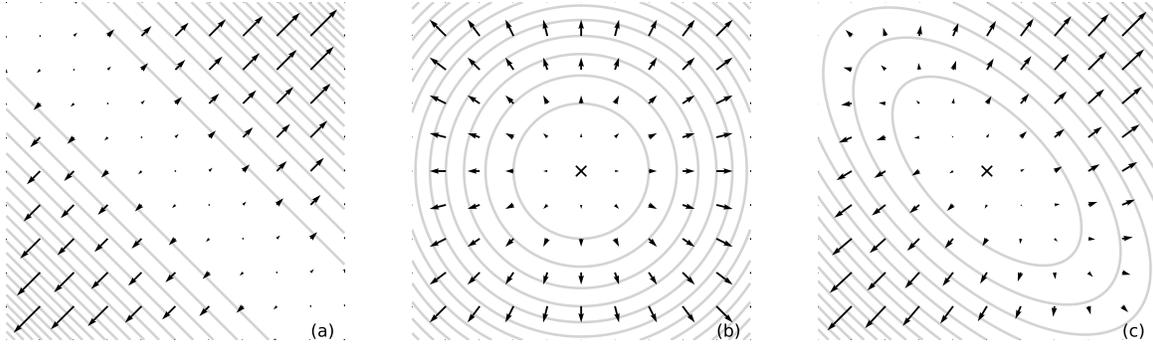
Figure 2: Examples of uniform areal recharge. Equipotentials (grey), discharge vectors (arrows), and high points (cross) for (a) straight equipotentials (linear recharge) for flow in direction  $\alpha = \pi/4$ , (b) circular equipotentials (circular recharge), and (c) elliptical equipotentials (elliptical recharge).
