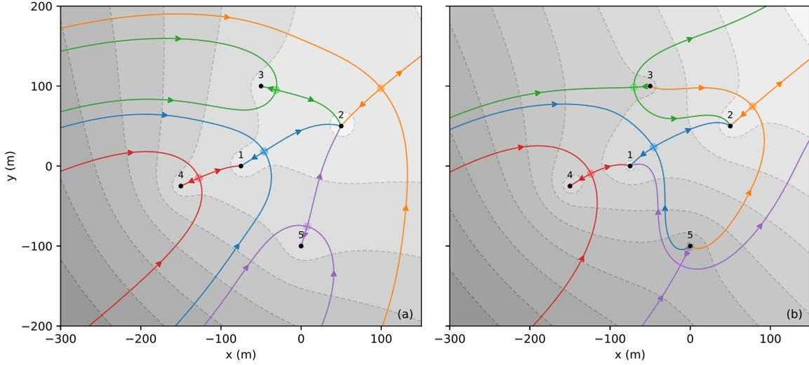
Figure 1: Example of five wells in uniform background flow. Equipotentials (filled grey contours, darker grey is higher potential), capture zone envelopes (colored), and stagnation points (light colored dots) for (a) Case 1 with five extraction wells, and (b) Case 2 with three extraction and two injection wells.
