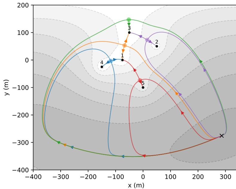
Figure 5: Examples of five wells (Case 1 in Table 1) in elliptical recharge background flow centered at  $(x, y) = (0, -200)$ . Equipotentials (filled grey contours, darker grey is higher potential), capture zone envelopes (colored), five saddle points (light colored dots), and one high point (cross).
