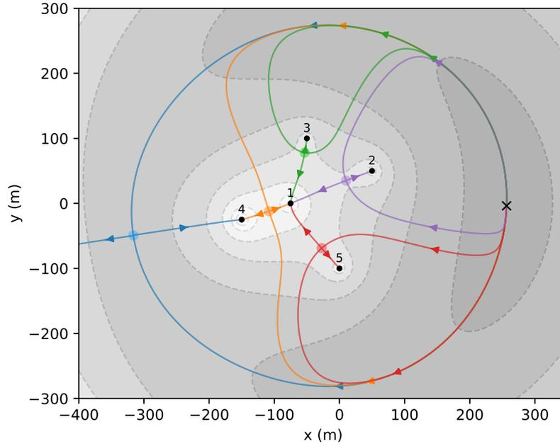
Figure 4: Examples of five wells (Case 1 in Table 1) in circular recharge background flow centered at the origin. Equipotentials (filled grey contours, darker grey is higher potential), capture zone envelopes (colored), five saddle points (light colored dots), and one high point (cross).
