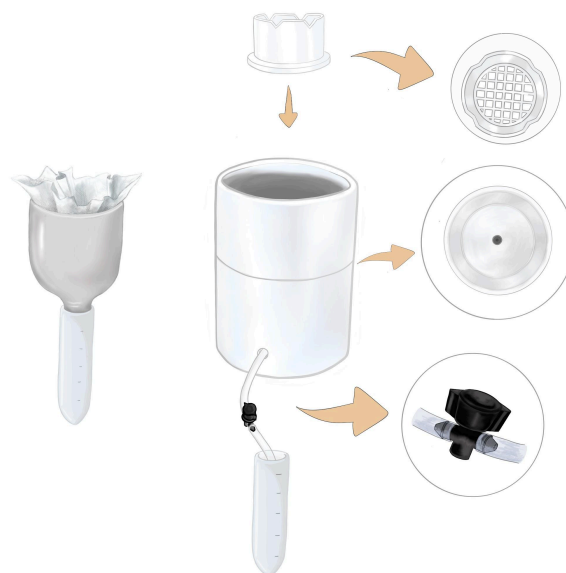
Figure 3. Bioassay 1 Illustration: The Baermann funnel (left), consists of a half-plastic bottle connected to a collecting tube and containing a single KimTech Science™ KimWipes™ serving as a filter paper. On the right is the NEMA Device, imitating the Baermann funnel, with the screen facing upwards to hold the filter paper and soil.
