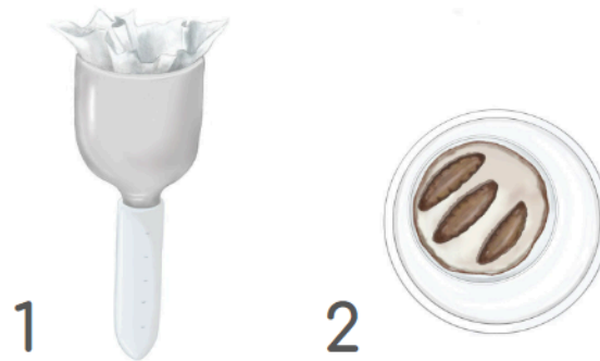
Figure 1. Traditional Methods Illustration: The Baermann funnel (1) for extracting nematodes from soil and the White trap (2) for multiplying/rearing nematodes.
