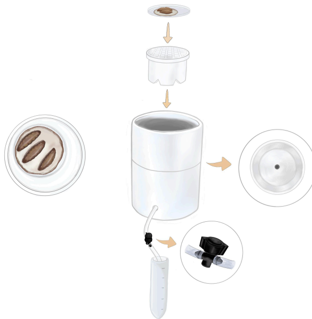
Figure 4. Bioassay 2 Illustration: On the left, the White trap method is shown, with a small Petri placed inside a medium Petri dish filled with reverse osmosis water. On the right, this aspect of the NEMA Device uses aspects of the White trap method, with the screen facing downwards and a small Petri dish placed on top.
