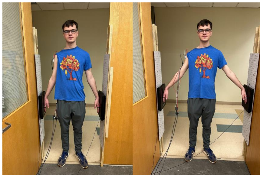
Figure 1. Standard position of the subjects during the experiment, showing [A] the narrow (1.0m) and [B] wide (1.5m) frame widths.
