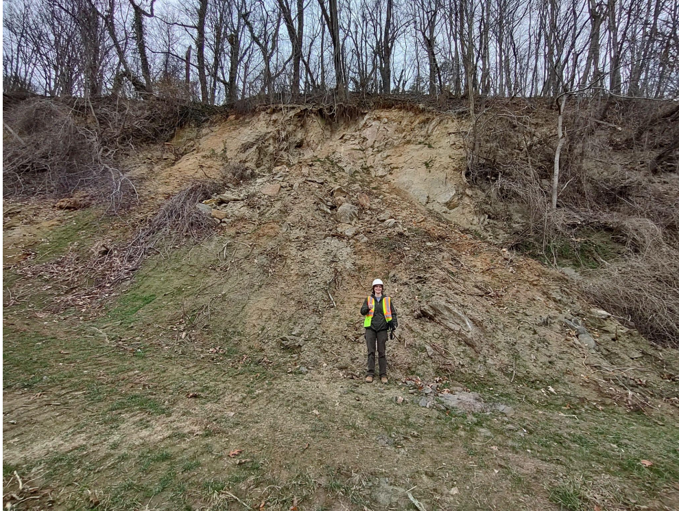
Figure 7. Field photo of the landslide indicated in figure 9. East facing wedge failure landslide that is located off of I-240 towards Knoxville, TN with a person for scale.
