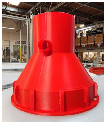
Figure 11. 3D printed IBC lid adapter first iteration.
