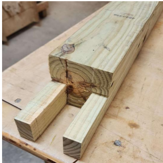
Figure 6. Joint design of side pieces for cradle prototype.
