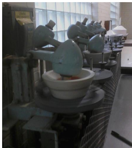
Figure 2.2.1 ii) Automated Pulverizing Machine, NC State University Minerals Research Laboratory in Asheville, NC
