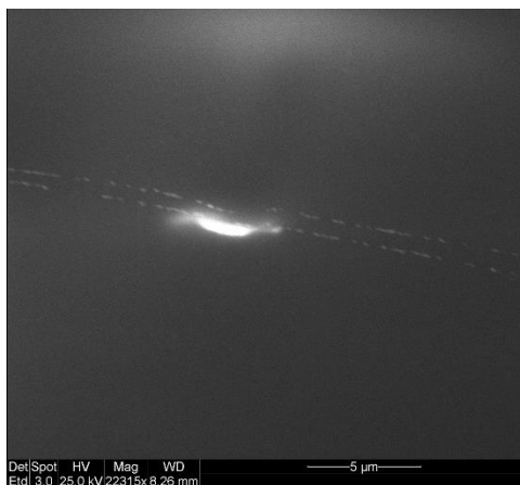
Image 8. SEM image of silver nanowires in PDMS.
