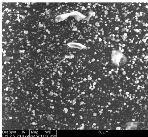
Image 7. SEM image of silver nanoparticles randomly dispersed in PDMS.
