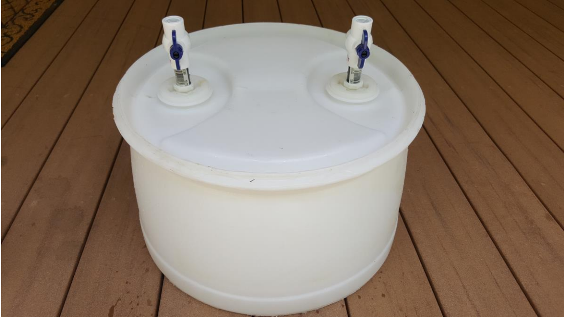
Figure 1. Seepage meter constructed to measure flow from lake bottom.
