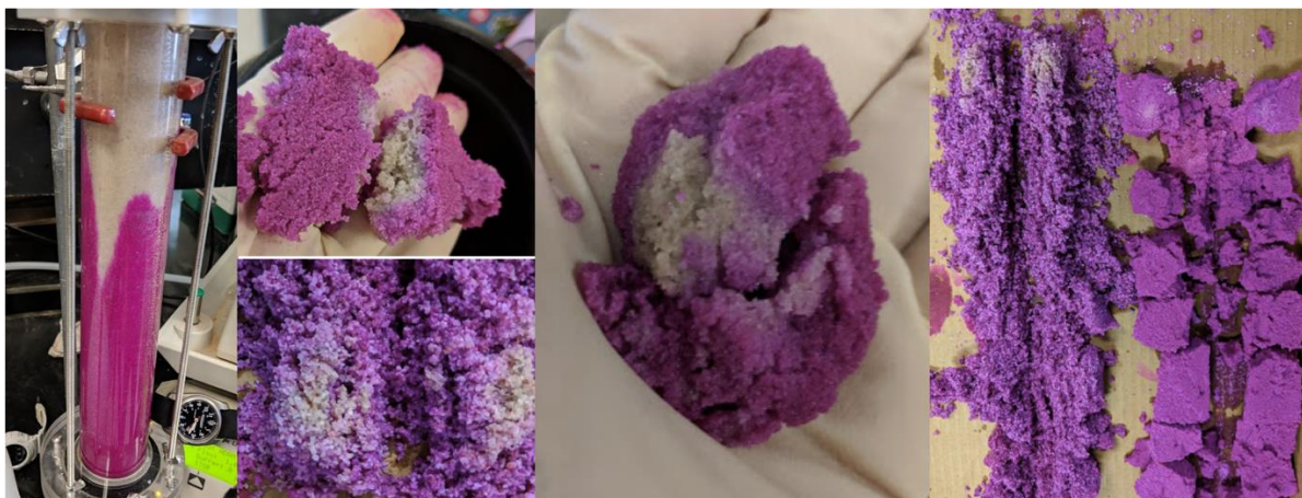
Figure 5. Dye tracer plume traveling in the column, voids found in 0.25-0.50mm grain size columns and 1-2mm grains size columns, split cross section of two soil columns
