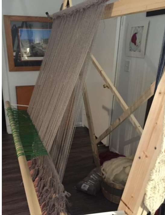
Fig. 2 shows the heddles in use, creating an open shed for the shuttle to pass through. All photos are my own, unless mentioned otherwise.
