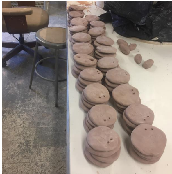
Fig. 3 shows the unfired clay weights, stacked and ready for the kiln.
