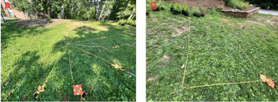
Figure 3. Set up for circle and square shapes, using meter tapes. A is a circle with a diameter of 4 m and a radius of 2 m. B is a 2 m x 3.6 m square.
