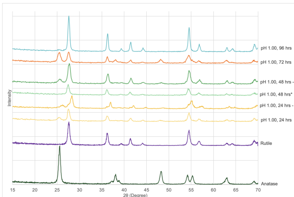
Figure 7. XRD Patterns of Purchased Anatase and Rutile, with Samples Synthesized at pH=1.00, second trial under the same condition marked with a dash (-)
