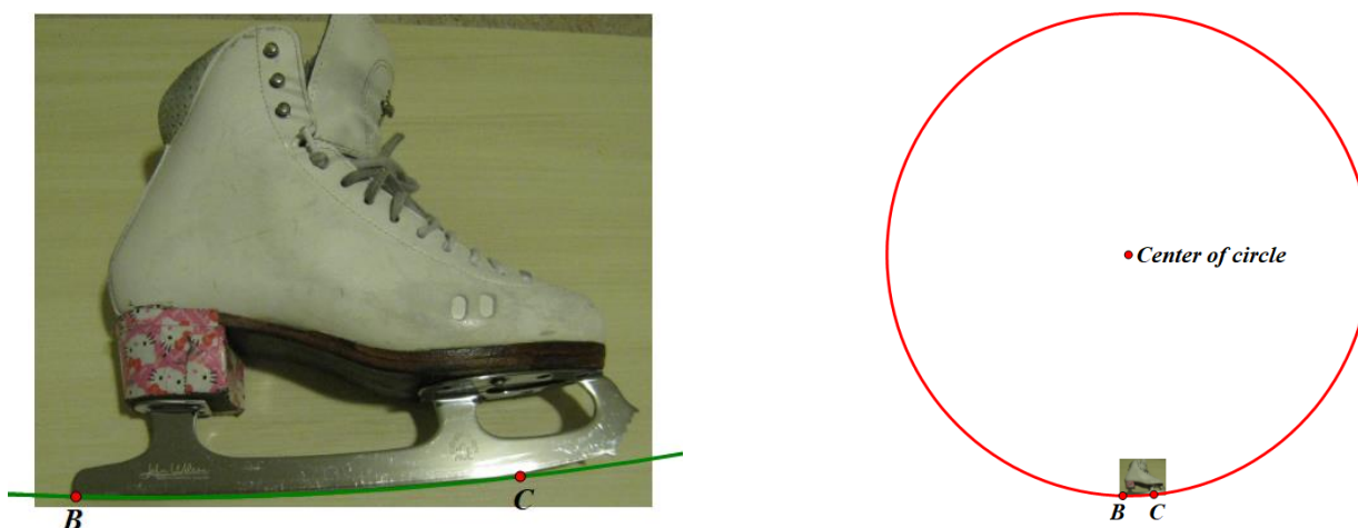
1 Figure 1. The figure skate blade has circular curvature.
